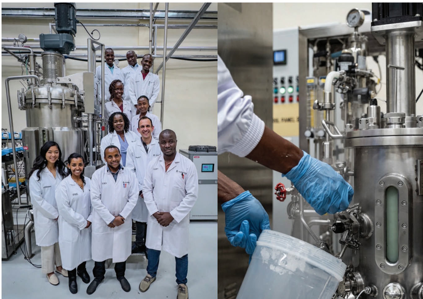
Left: Essential's biosciences facility is located in Mlolongo, just outside Nairobi County, with a team comprised of 13 members. Right: Essential's biomanufacturing process includes transferring the seed produced in this 20 L bioreactor into our 700 L bioreactor. Photo credits: Essential
