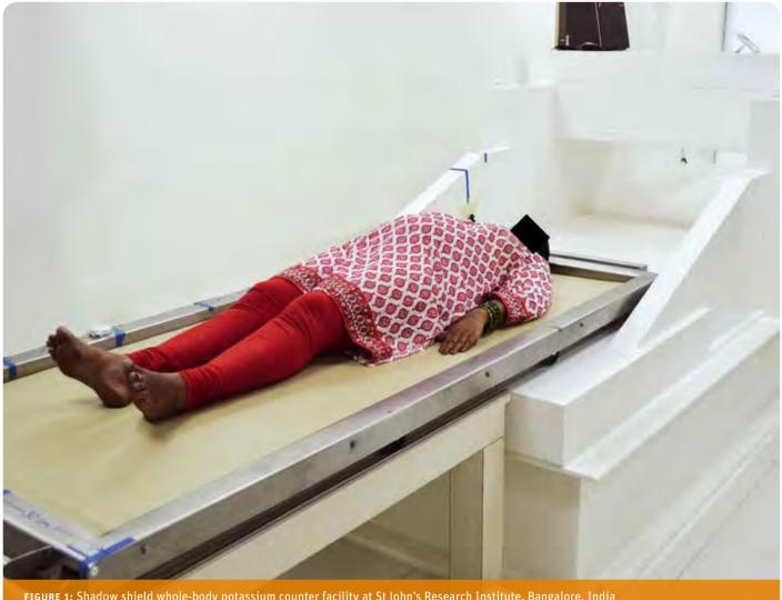
FIGURE 1: Shadow shield whole-body potassium counter facility at St John's Research Institute, Bangalore, India
